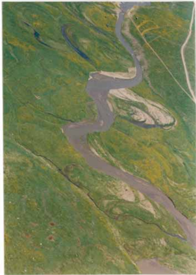
Figure 13. Weminuche River in Colorado (C4 stream type) showing change in channel stability, pattern, dimension, and bank erosion due to a willow/grass conversion.
